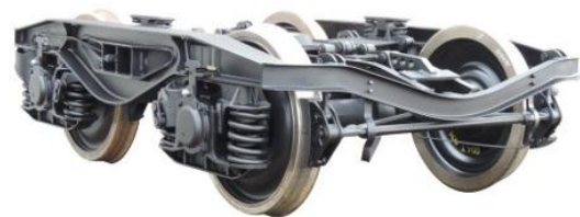
Fig. 1. Illustration of the original Y25 bogie design
