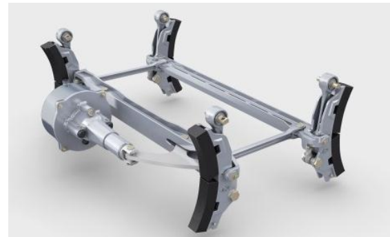
Fig. 3. Integrated block brake for goods wagons [10]
