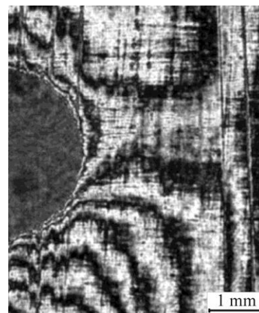
Fig. 4. Interference map in the vicinity of the stress concentrator without a crack in the 7075-T6 aluminum alloy specimen
