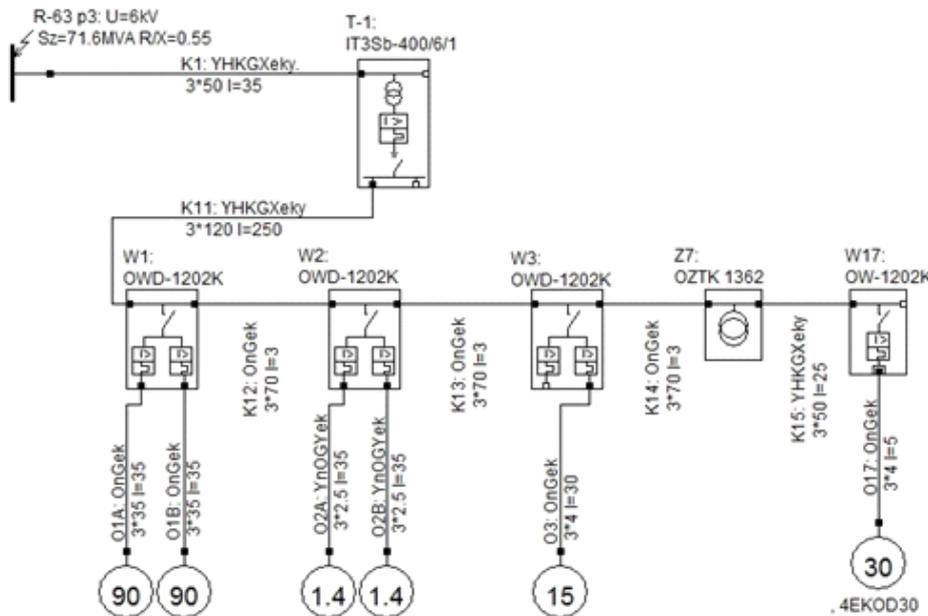
Fig. 1. Electric scheme of analyzed conveyor belt [12]
