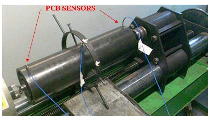
Fig. 3. Test stand with mounted roller and accelerometers
