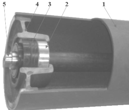
Fig. 1. The construction of belt roller:
