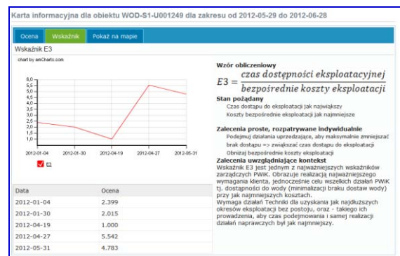
Fig. 16. The ISSOE screen with example single measure visualization of the analysis results [21]
