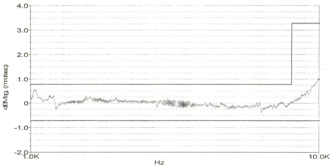
Figure3. Characteristics of the vibration sensor (range 1 000 - 10 000 Hz).
