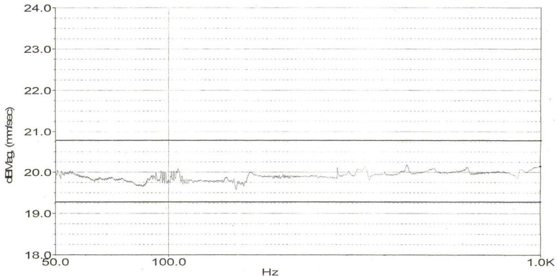
Figure. 2. Characteristics of the vibration sensor (range 50 - 1 000 Hz).
