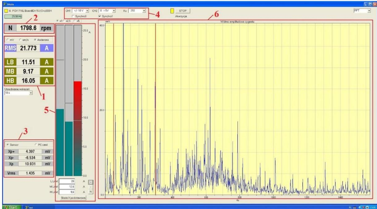
Fig 5. The main software interface ANDEROMETER: 1 noise indicators, 2-spindle speed, 3-voltage, 4- measuring range of the measuring card, 5- analog indicators of the noise floor, 6-amplitude spectrum.
