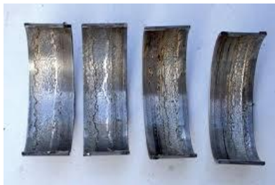
Fig. 1. Typical types of cavitation parts` wear
