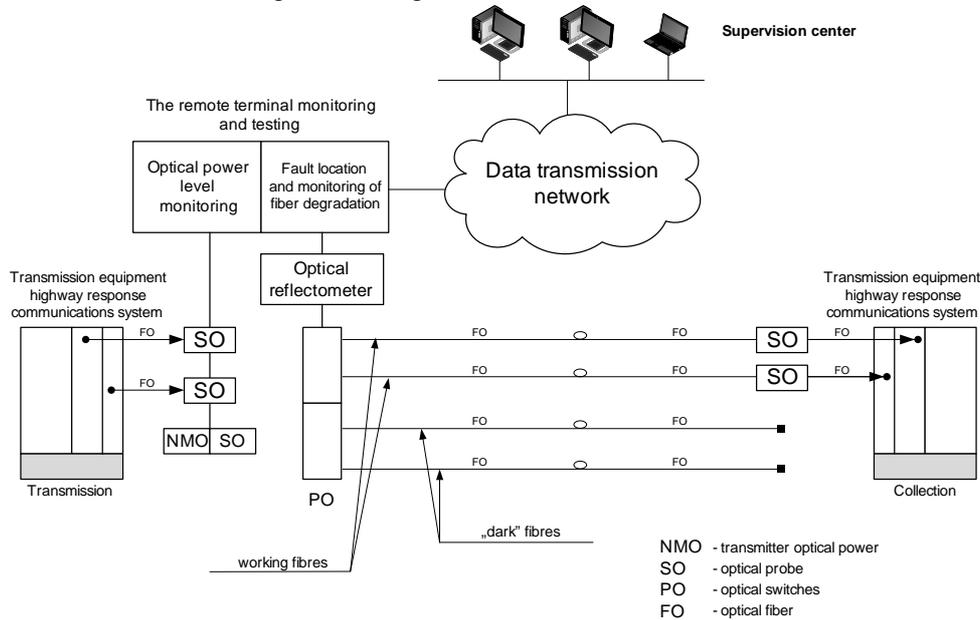
Fig. 2. Scheme of the automatic control of optic fibres
