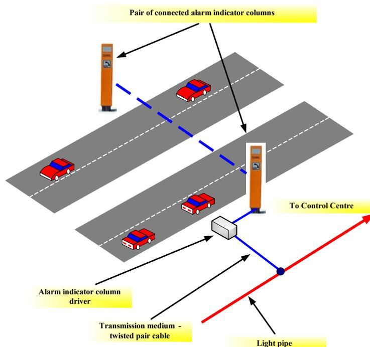
Fig. 1. Architecture of the highway emergency response system
