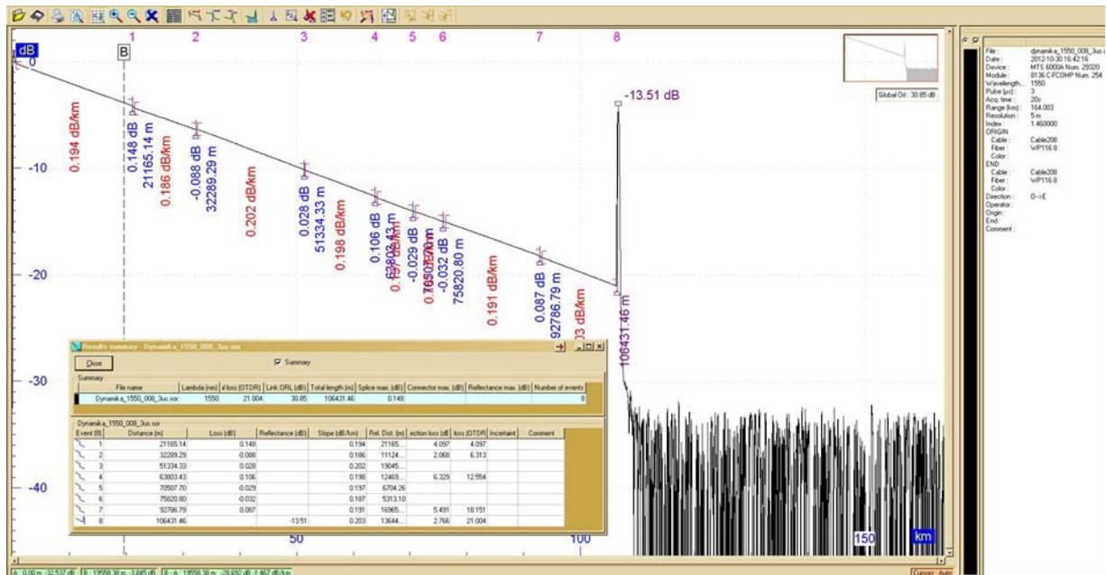
Fig. 3. Reflectometric measurement of the tested fibre optic track [15]
