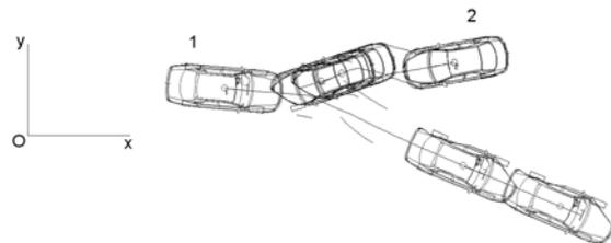
Fig. 3. The coordinate system Oxy for oblique frontal collision. Vehicles during collision along with the deformation of their bodies shown, where 1 - Audi, 2 - Mazda
