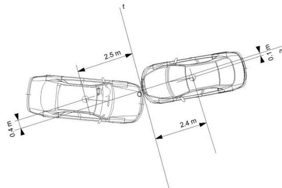
Fig. 4. Location of the vehicles in the local coordinate system for the frontal oblique impact
