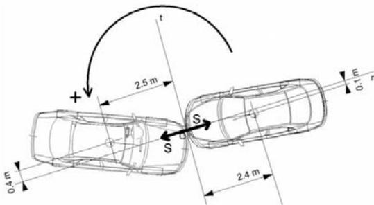
Fig. 5. The positive direction of the angle measurement relative to the x-axis of the global coordinate system and the angle of inclination of the translational velocity relative to the x axis
