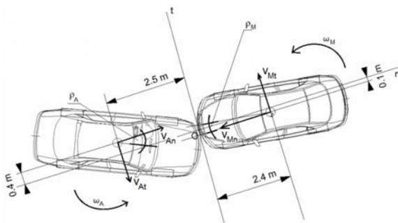
Fig. 6. Velocity components and angular velocities at the moment of collision. Also the distances from the center of the mass of each vehicle to the origin of the local coordinate system Ont are indicated
