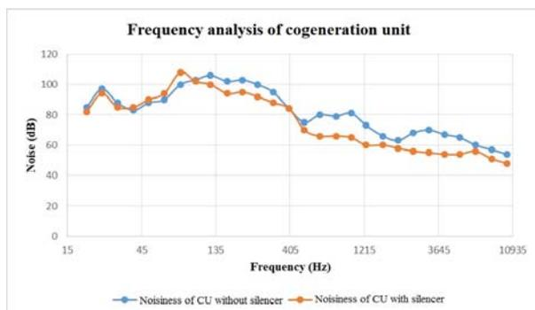
Fig. 16: Graph of the frequency analyse
