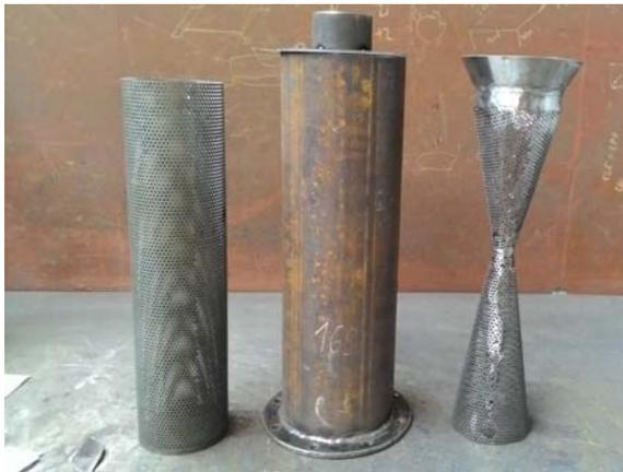
**Fig. 10:** Parts of muffler
