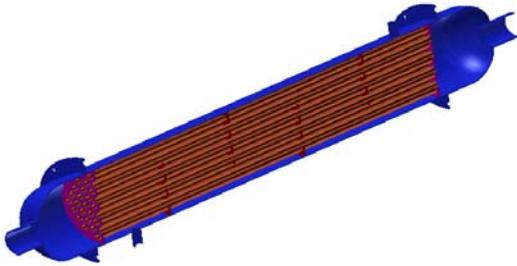
**Fig. 1:** 3D model of designed exhaust gas exchanger
