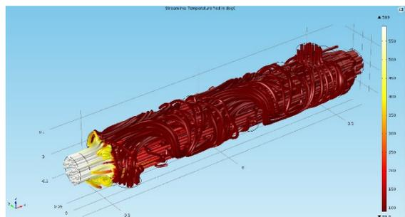
**Fig. 6:** Streamline in the exhaust gas heat exchanger
