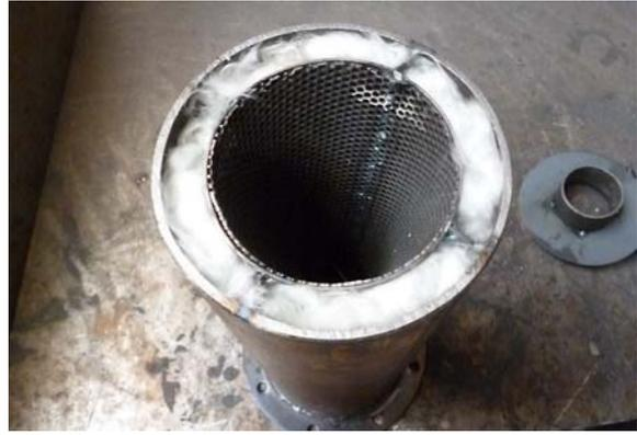
**Fig. 11:** Glass wool inside of muffler
