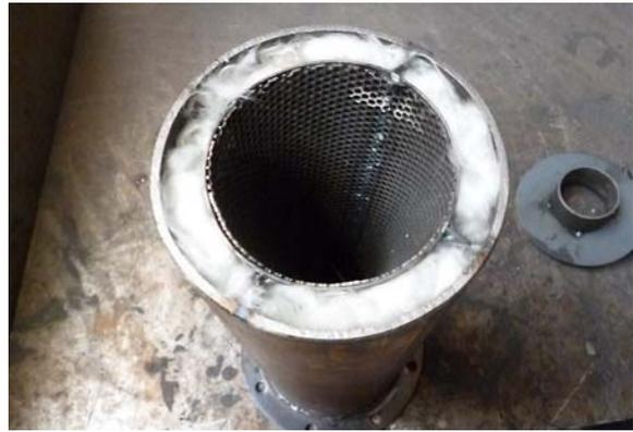
**Fig. 11:** Glass wool inside of muffler
