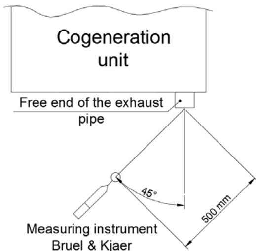
Fig. 15: Measurement scheme
