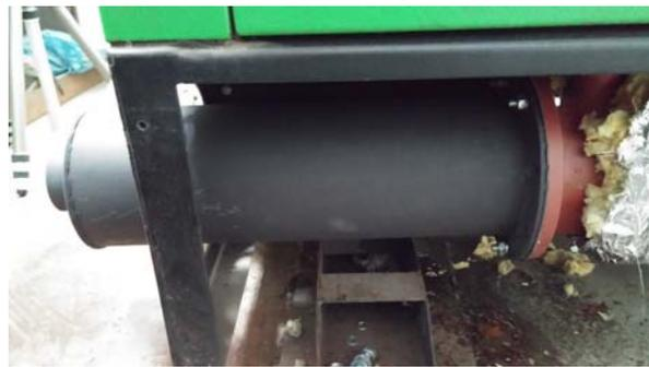
**Fig. 13** The muffler mounted on the heat exchanger
