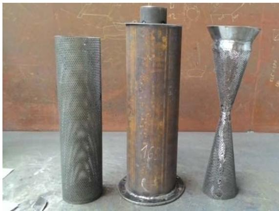
**Fig. 10:** Parts of muffler
