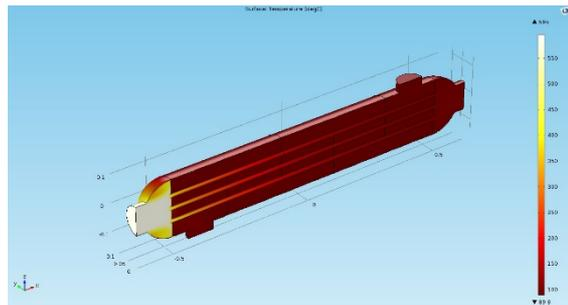
**Fig. 5:** Temperature of the exhaust gas heat exchanger in °C [6]
