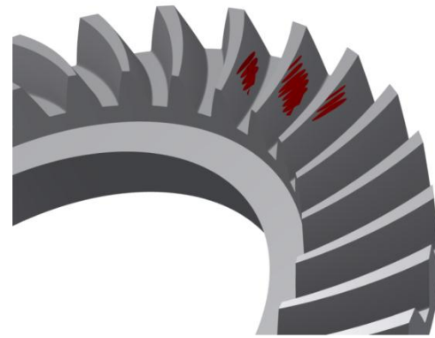
Fig 2. Summary bearing on the gear tooth flank
