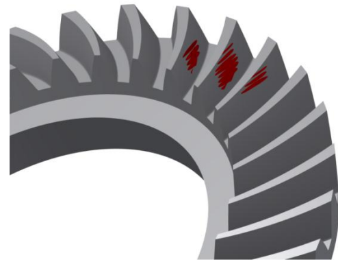
Fig 2. Summary bearing on the gear tooth flank
