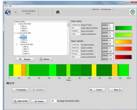
Fig. 8. Visualization of test results using Diagbelt system
