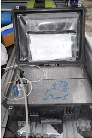
Fig. 5. Belt Guard recorder from Australian company Beltscan
