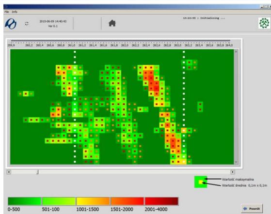
Fig. 10. Image of a damaged or defectively performed splice
