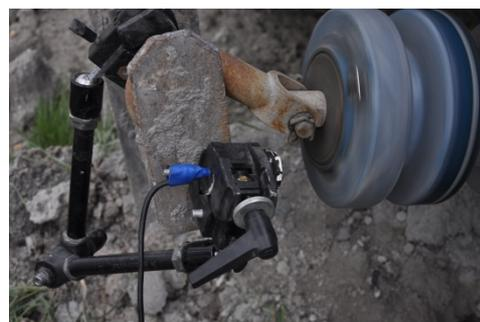
Fig. 4. Measurement of conveyor velocity with magnetic encoder
