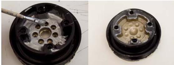
Fig. 12. Optically active layers adhered on the model of the torsion vibration damper in justified cases
