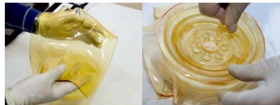
Fig. 9. Process of applying an optically active layer of real torsional vibration damper made of resin and the casting method
