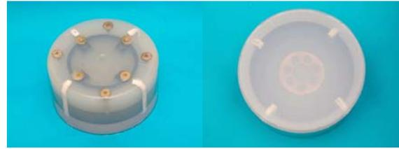
Fig. 4. The silicone mold of torsional vibration damper after completion of the curing process
