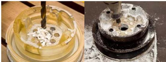
Fig. 13. Drilling of holes in the optically active layers
