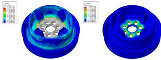
Fig. 17. Distribution effort of in the area of a damper hub mounting obtained by MES
