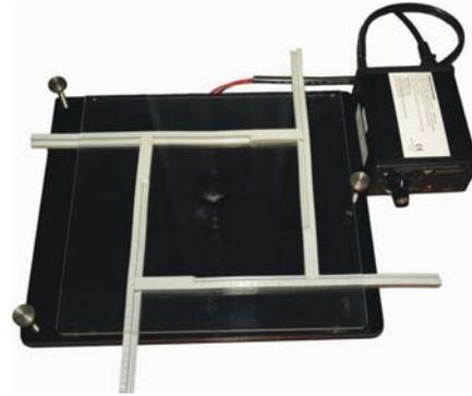
Fig. 8. Teflon plate for producing an optically active layer
