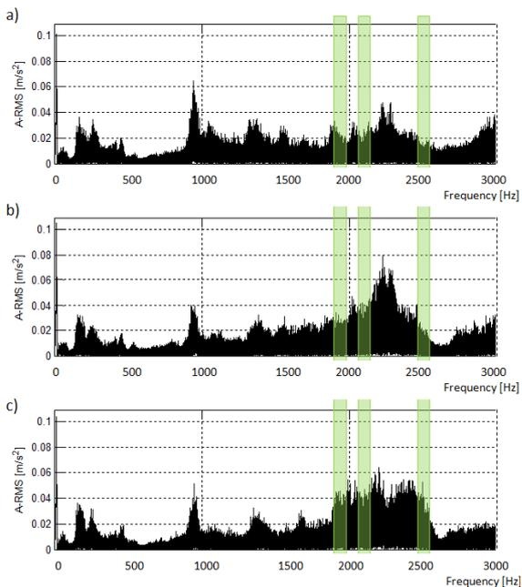
Fig. 6. Dependence of amplitude of vibration accelerations on frequencies for different pad's thicknesses during braking from speed of 160km/h in direction  $YI$ : a) pad's thickness  $G1=35\text{mm}$ , b) pad's thickness  $G2=25\text{mm}$ , c) pad's thickness  $G3=15\text{mm}$
