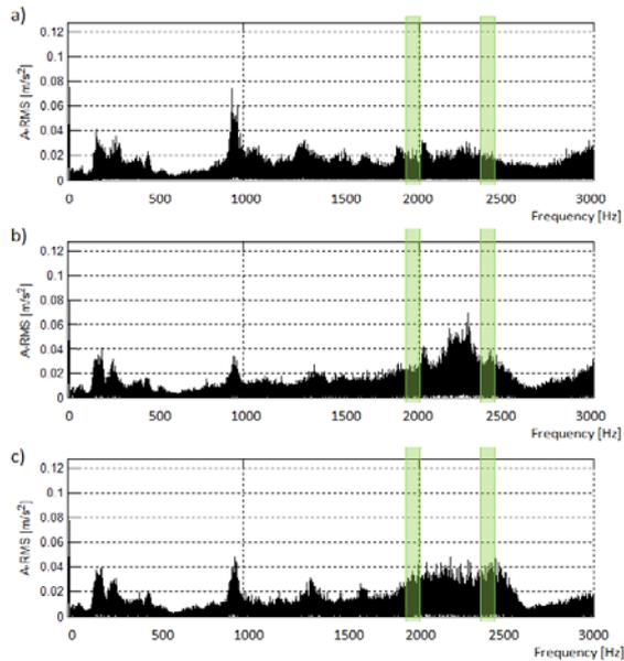
Fig. 5. Dependence of amplitude of vibration accelerations on frequencies for different pad's thicknesses during braking from speed of 120km/h in direction  $YI$ : a) pad's thickness  $G1=35\text{mm}$ , b) pad's thickness  $G2=25\text{mm}$ , c) pad's thickness  $G3=15\text{mm}$
