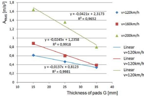
Fig. 9. Dependence of pad's thickness in function of point parameters ( $A_{RMS}$  value) of vibrations accelerations for measurement in the  $Y_1$  direction for speed at the beginning of braking  $v=120, 160$  and  $200\text{km/h}$
