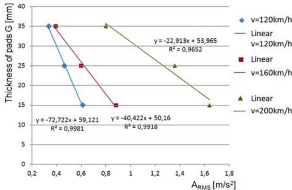
Fig. 10. Dependence of pad's thickness in function of point parameters ( $A_{RMS}$  value) of vibrations accelerations for measurement in the  $Y_1$  direction for speed at the beginning of braking  $v=120, 160$  and  $200\text{km/h}$
