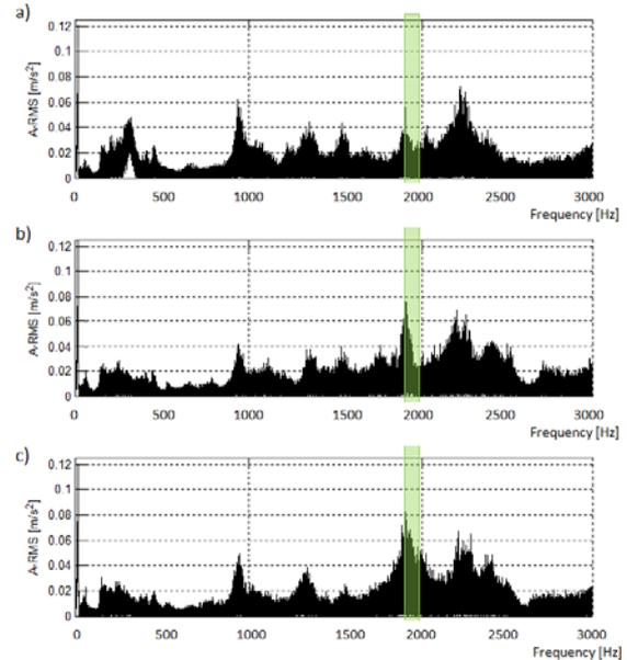
Fig. 7. Dependence of amplitude of vibration accelerations on frequencies for different pad's thicknesses during braking from speed of 200km/h in direction  $YI$ : a) pad's thickness  $G1=35\text{mm}$ , b) pad's thickness  $G2=25\text{mm}$ , c) pad's thickness  $G3=15\text{mm}$
