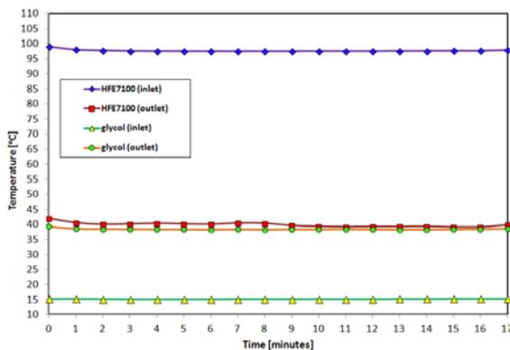
Fig. 5. The temperatures of the HFE7100 and glycol in the condenser vs. time
