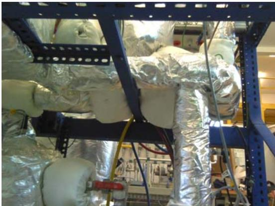
Fig. 10. The photo of the tested evaporator
