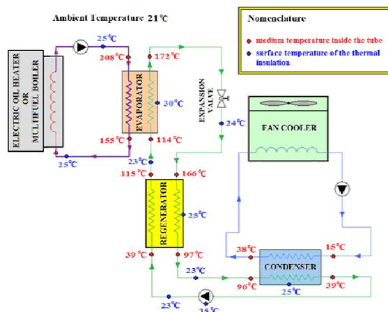
Fig. 20. Scheme of the ORC installation with provided temperature values of the working media
