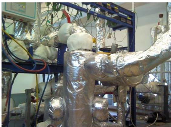
Fig. 18. The droplet separator for the HFE7100
