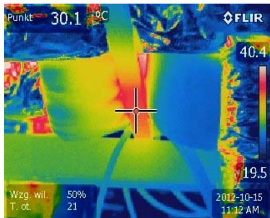
Fig. 11. The thermal image of the evaporator
