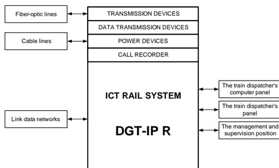
Fig. 1. The general structure of the KST DGT-IP R system
