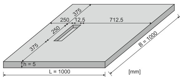
Fig. 1. Geometry of tested steel plate with damage
