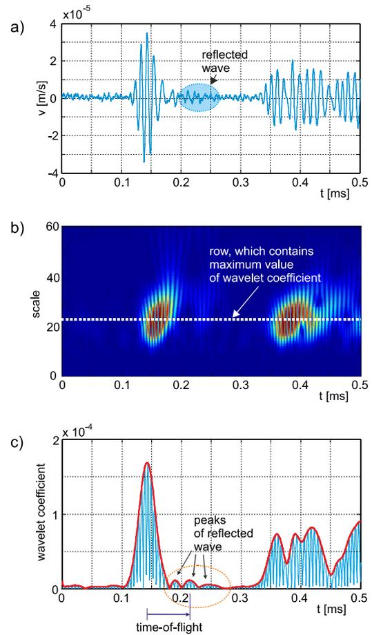
Fig. 5. The wavelet procedure of identification of reflection from damage: a) time signal of propagated Lamb wave; b) scalogram for continuous wavelet transform for scale  $s = 22$ ; c) envelope of selected wavelet coefficient
