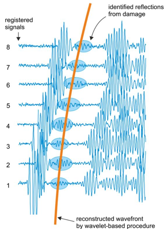
Fig. 9. Reconstructed shape of the wavefront reflected from damage by wavelet-based procedure
