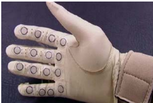
Fig. 2. Finger force measurement system (volar side) [3]
