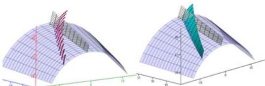
Fig. 5. Grid of points (left-hand drawing) representing the numerical solution to the envelope equation (1.1) – defining the convex surface of pinion tooth flank (the right-hand drawing shows the interpolated surface)
