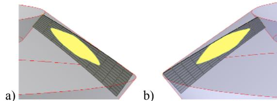
Fig. 8. Reference summary contact pattern for a 18:43 transmission on the drive side (a) and coast side (b) of the left-hand gear generated on the basis of data presented in Tables 1, 2 and 3
