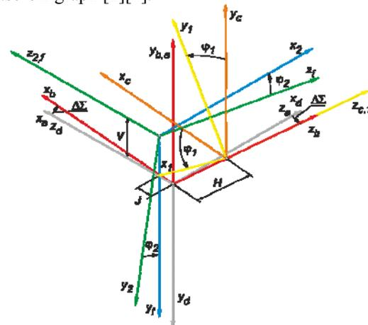
Fig. 3. Design gear model with deviations as applied: in the analysis of the effect of tooth geometry on gear meshing quality (for zero deviations); and to determine the gear's sensitivity to assembly and manufacturing errors
