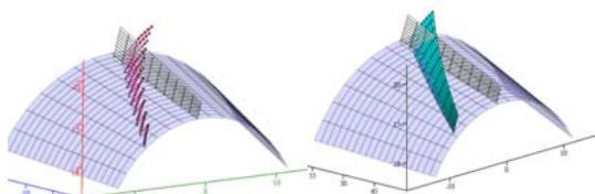
Fig. 5. Grid of points (left-hand drawing) representing the numerical solution to the envelope equation (1.1) – defining the convex surface of pinion tooth flank (the right-hand drawing shows the interpolated surface)
