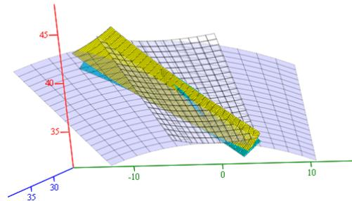
Fig. 7. Momentary gear contact pattern (yellow – pinion, turquoise – gear, other parts of pinion and gear reference cones)
