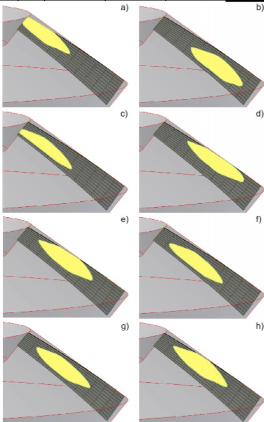
Fig. 10. Summary contact patterns for a 18:43 transmission on the drive side of the gear tooth (left-hand gears) for the assumed deviations (positive and negative) V, H, J and  $\Delta\Sigma$
