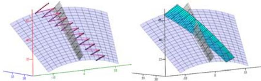
Fig. 4. Grid of points (left-hand drawing) representing the numerical solution to the envelope equation (1.1) – defining the concave surface of gear tooth flank (the right-hand drawing shows the interpolated surface)
