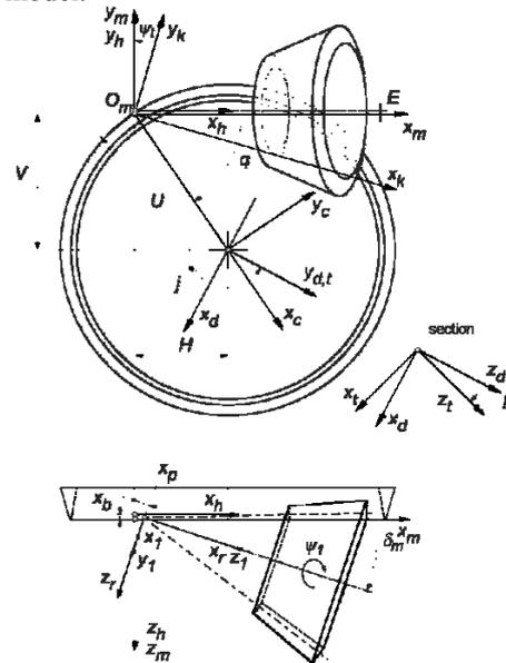
Fig. 1. The location of the machined gear in the technological model together with a set of coordinate systems for machine tool subassemblies reflecting the set-up of technological parameters
