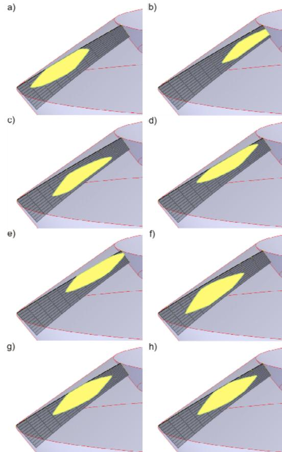
Fig. 11. Summary contact patterns for a 18:43 transmission on the coast side of gear tooth (left-hand gears) for the assumed deviations V, H, J and  $\Delta\Sigma$ .
