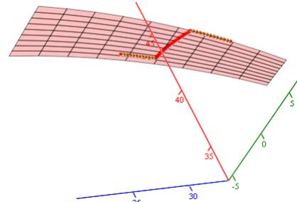
Fig. 6. Contact path illustrated on the concave surface of the gear flank
