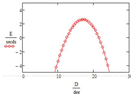
Fig. 9. Transmission error graph
