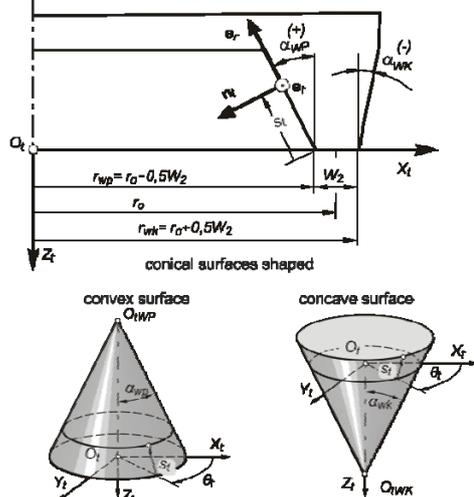
Fig. 2. Geometry of conical surfaces forming concave and convex tooth flanks [6]
