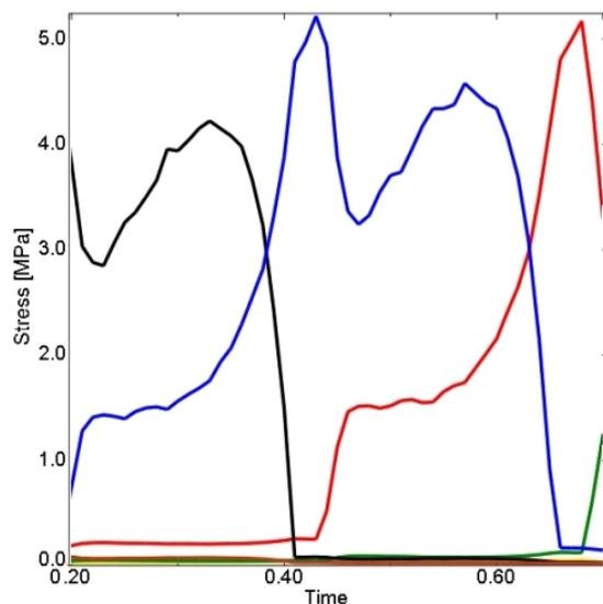
Fig. 8. The pattern of bending stress variation  $\sigma_z$  at roots of subsequent mating teeth of pinion no 1
