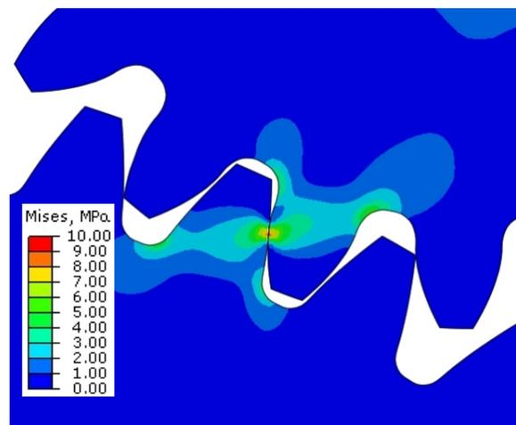
**Fig. 4.** Distribution of reduced stress for one-pair teeth mating of the gear with pinion no2
