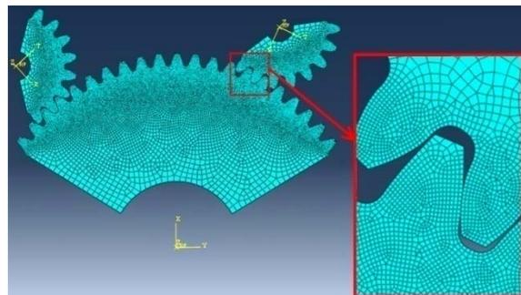
Fig. 1. Models of wheels in the dual-path gearing ready for FEM computation
