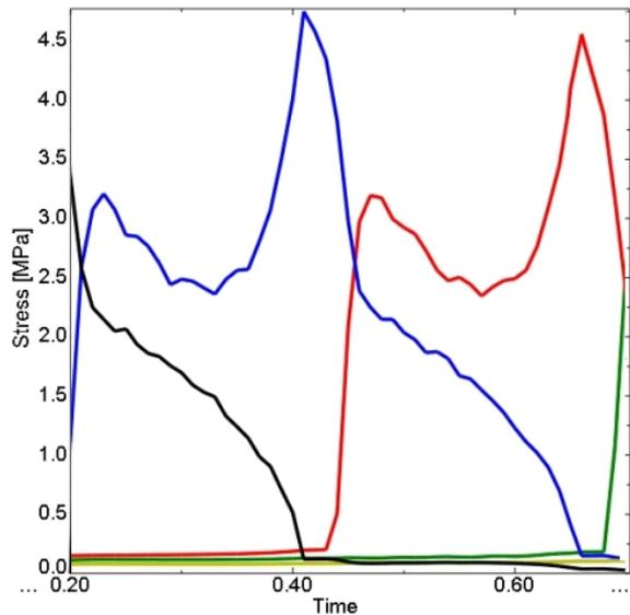
Fig. 7. The pattern of bending stress  $\sigma_z$  at roots of selected teeth of the gear
