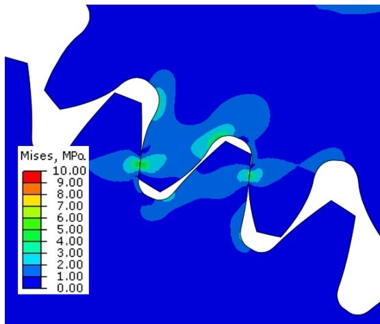
Fig. 6. Distribution of reduced stress for two-pair teeth mating of the gear with pinion no2
