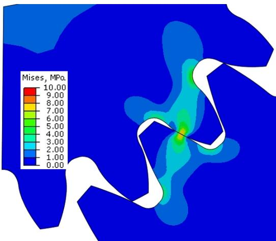
**Fig. 3.** Distribution of reduced stress for one-pair teeth mating of the gear with pinion no 1
