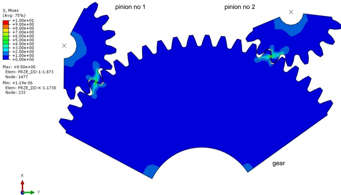
**Figure 2** Distribution of reduced stress [MPa], in wheels of dual power-path gearing obtained by FEM computation in Abaqus.
