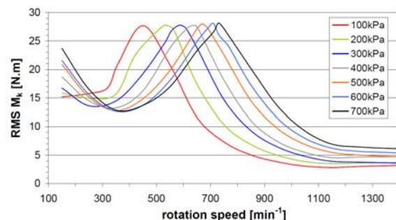
Fig. 3. Resonant curves of the mechanical system at various air overpressure in the tuner  $p_{PS}$
