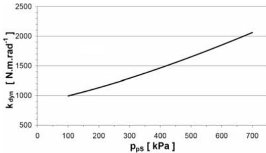
Fig. 4. Dynamic torsional stiffness of the tuner  $k_{dyn}$  dependent on overpressure  $p_{ps}$  in the tuner
