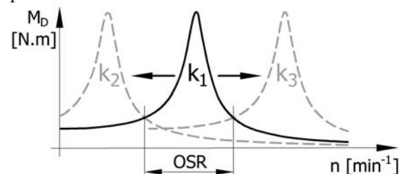
Fig. 1. Mechanical system tuning principle
