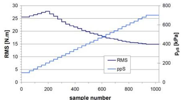
Fig. 7. Example of searching a local minimum of objective function of the mechanical system by the electronic extremal control system MESLER at mechanical system rotation speed  $500 \text{ min}^{-1}$
