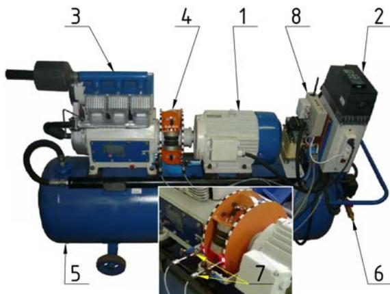
Fig. 2. Implemented torsional oscillating mechanical system
