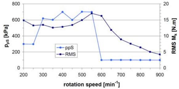
Fig. 6. Optimal air overpressure  $p_{ps}$  and RMS  $M_k$  value in relation to the rotation speed of mechanical system
