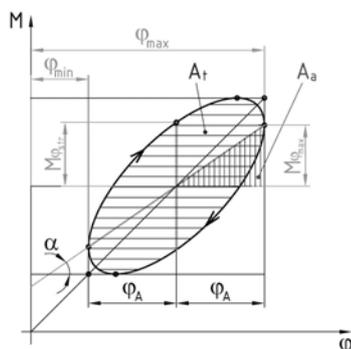
Fig. 2 Example of evaluation of the hysteresis loop
