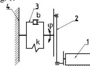
Fig. 1 Kinematic scheme of measuring with brake mass
