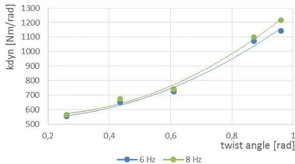
Fig. 5 Dependence of dynamic stiffness on a preload and on two oscillation frequencies
