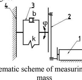
Fig. 1 Kinematic scheme of measuring with brake mass
