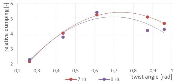
Fig. 6 Dependence of the relative damping on the preload and oscillation frequency
