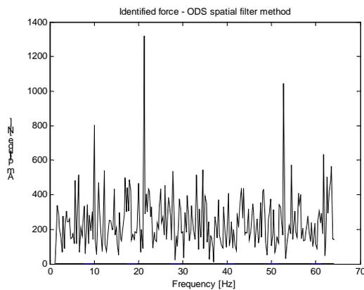
Fig. 4. Excitation force identified with use of spatial filter based on ODS
