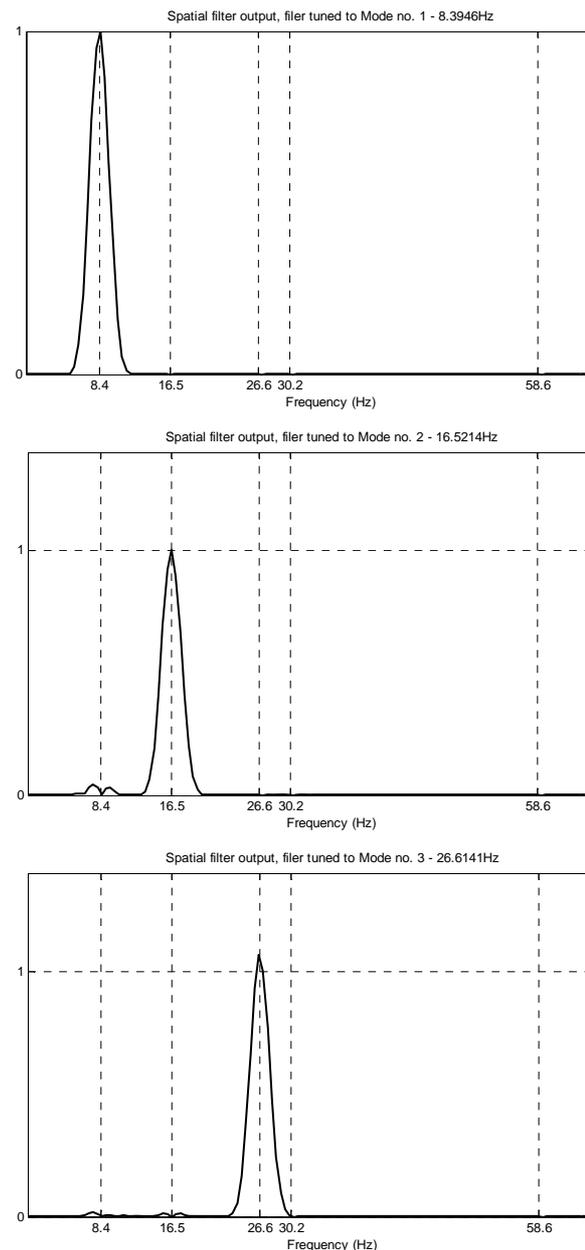
Fig. 3. First three outputs of spatial filter tuned for ODS corresponding to natural frequency of the system
