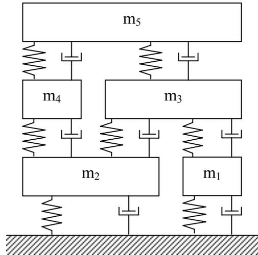
Fig. 1. Model used for simulation
