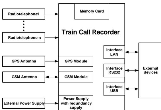
Fig. 1. General block diagram of train call recorder
