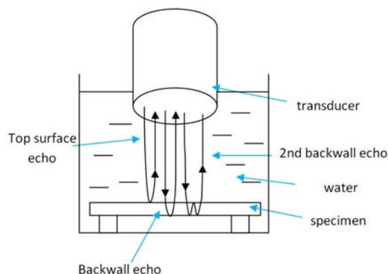
Fig. 1. Echo reflections in the specimen in immersion test
