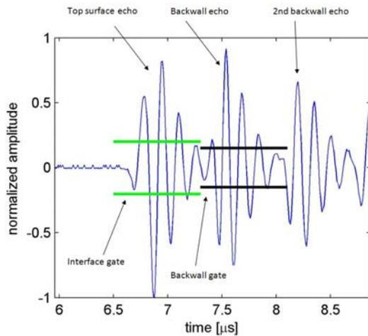
Fig. 2. A-scan with gates
