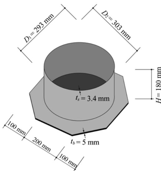
Fig. 1. Geometry of laboratory model of steel tank
