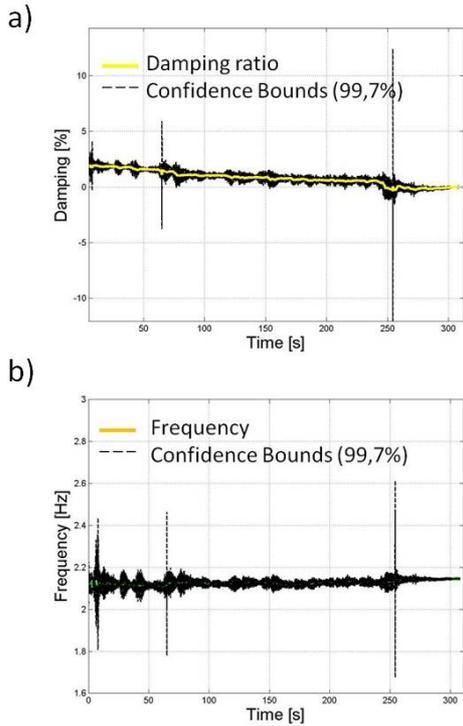
Fig. 6. Identified time history of modal parameters non – stationary aero - elastic system with estimated confidence bounds: a) damping ratio, b) natural frequency
