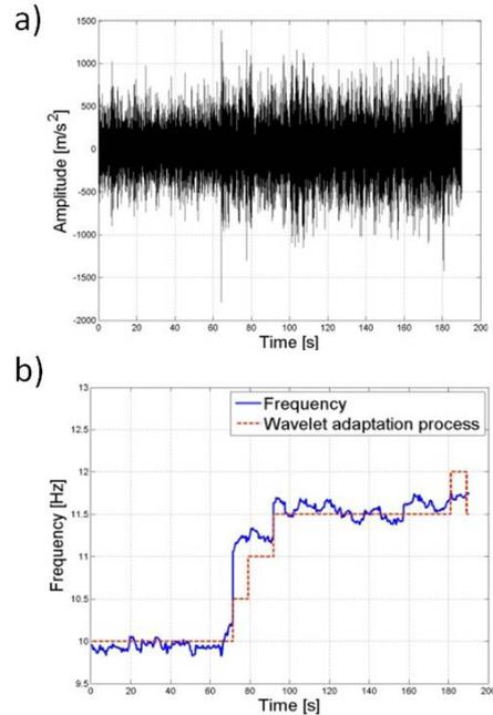
Fig. 8. System response (a), Comparison of identified natural frequency of the system (b)
