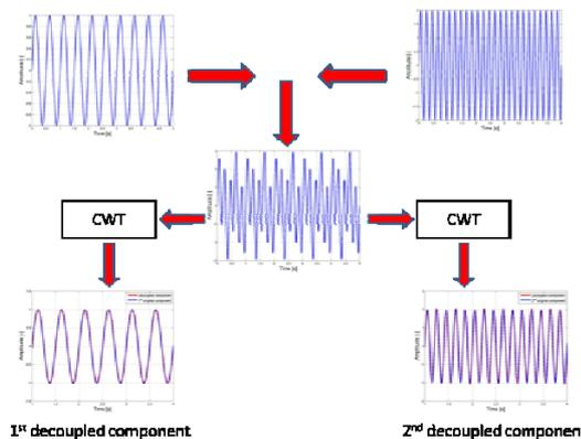
Fig. 2. Wavelet based signal components decoupling
