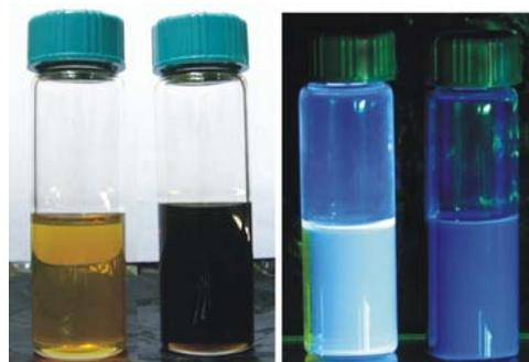
Fig. 1. Lubricating oil *Titan Truck Plus 15W40* - fresh and used (593 h) - in visible light (left) and in ultraviolet (right)
