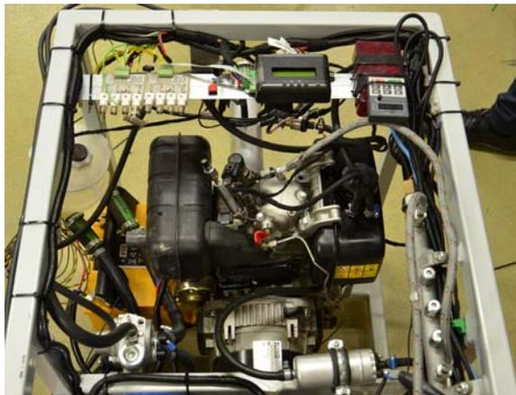
Fig. 1. Test stand with integrated modified engine
