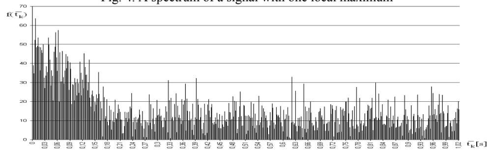
Fig. 5. A cepstrum of a signal with one local maximum
