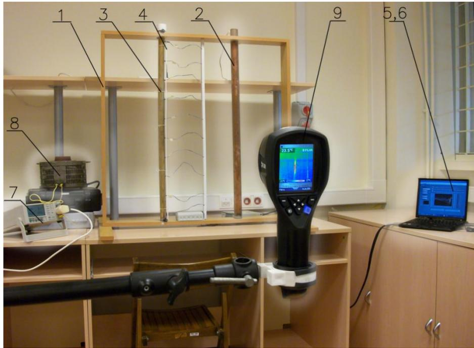
Fig. 3. Laboratory stand for determination of heat emission
