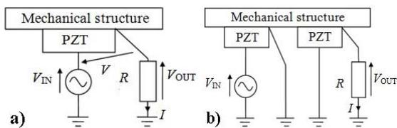
Fig. 1. Measurement of point FRF (a), and transfer FRF (b) of electromechanical impedance
