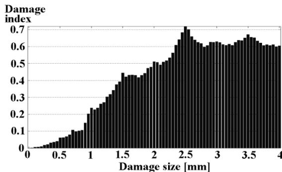
Fig. 10. Relationship between notch depth and damage index
