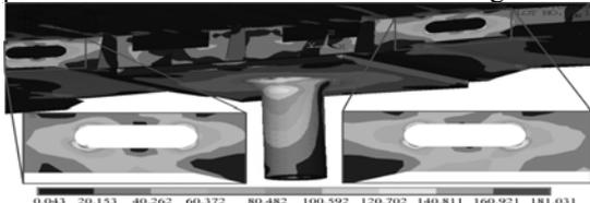
Fig. 5. Strain distribution (Von-Misses) [MPa]
