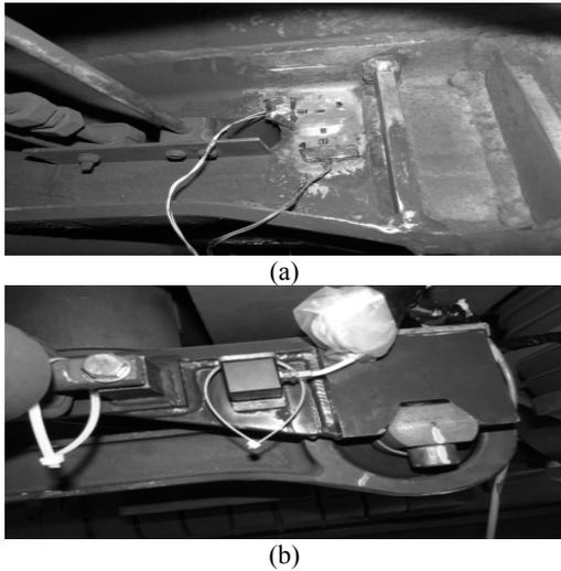
Fig.3. Location of sensors - (a) strain gauges, (b) tri-axial accelerometer
