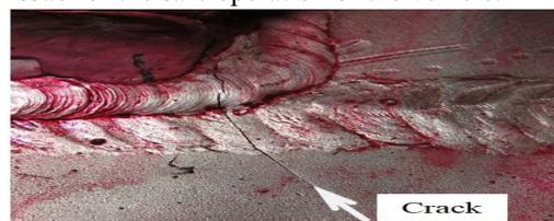
Fig.7. Cracks on a bolster beam of a Metro system
