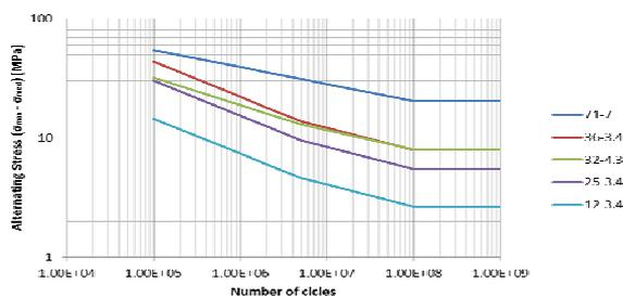
Fig.11. Whöler curves for different weld joint categories [15]
