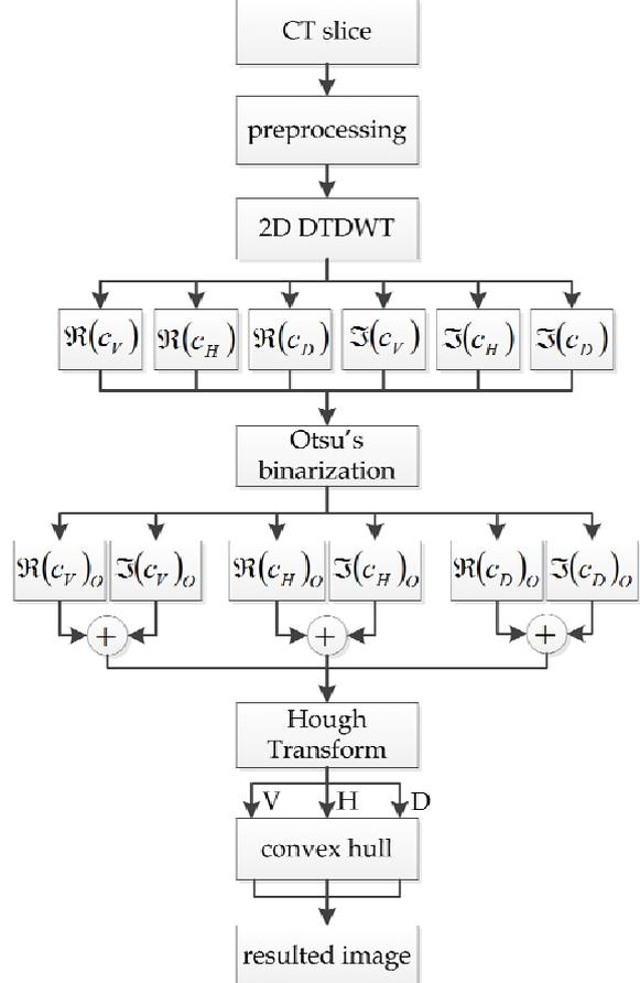
Fig. 2. Algorithm of directionality detection based on wavelet and Hough transforms
