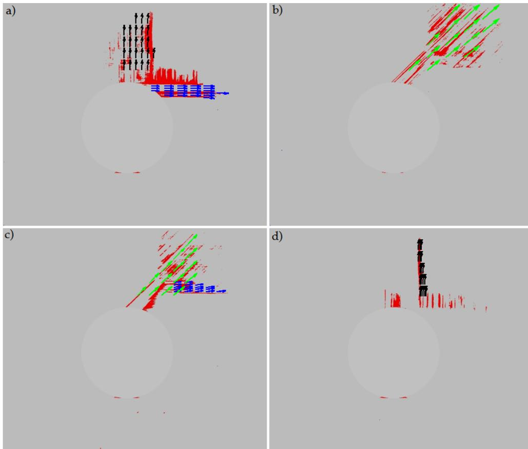
Fig. 5. Results of four different CT slices – detection of vertical, horizontal and diagonal directionality of delamination
