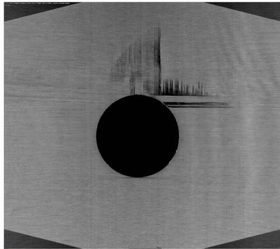
Fig. 1. Exemplary CT slice (cross section) of the carbon fibre composite specimen)
