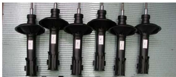
Fig. 6. Six examined front hydraulic shock absorbers
