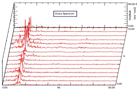
Fig. 8. CP plots (waterfall) for investigated points 1-15, respectively, operational modal analysis, impact excitation attached to the right pillar, in 2012
