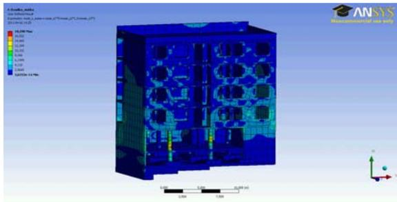
Fig. 15. Distribution of the sum of particular stresses for FE model
