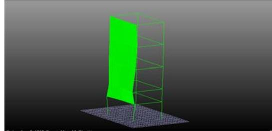
Fig. 4. The example of a mode shape of an identified natural frequency - 7,50 Hz for impact excitation attached to the left pillar in 2012
