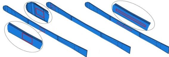
Fig. 6. Placement and shape of PZT patches
