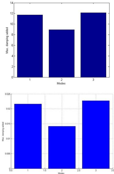
Fig. 5. Comparison between theoretical maximum added damping in terms of modal damping (Bottom) and actual decrease in response amplitude in dB (Top) for the third shape of the piezo patch
