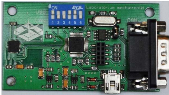
Fig. 3 Magnetic field and acceleration sensor board
