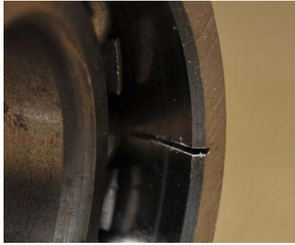
Fig. 6. Evolution of rolling bearing degradation with artificial defect on the outer raceway after its operation under loading of 14 N
