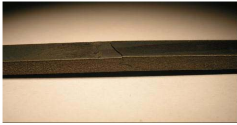
Fig. 2. Photograph of a fatigue-fractured sample of construction steel
