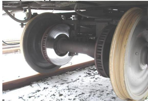
Fig. 1. View of two friction set mounted on axle passenger car
