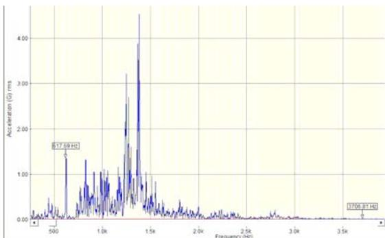
Fig.9. Vibration signal spectrum of the turbocharger in frequency range from 0 kHz to 4 kHz – magnetic sensor holder – engine no. 1
