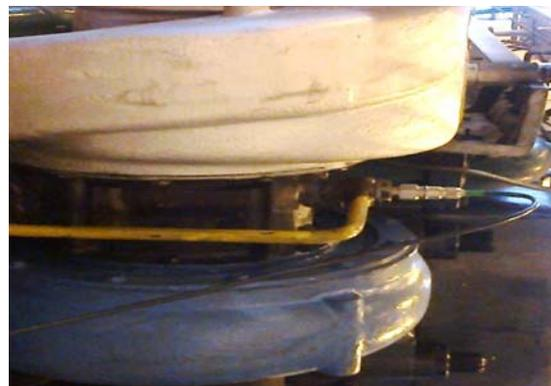
Fig. 11. Napier C–045/C type turbocharger with vibration sensor mounted on the bearing housing – engine no. 2
