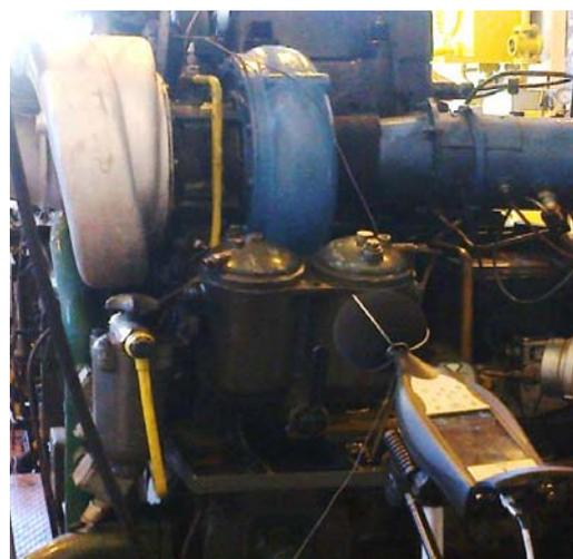
Fig. 3. Napier C-045/C type turbocharger with vibration sensor mounted on the bearing housing and 2250 B&K analyzer
