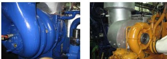
Fig. 1. PBS Turbo PDH-35 type axial-flow turbocharger on SULZER main engine type 8AL25/30 (left) and NAPIER C-045/C radial-flow turbocharger on SULZER auxiliary engine type 6AL20/24 (right)
