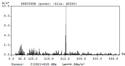
Fig. 3. Turbocharger amplitude of vibrations accelerations in frequency domain Main Engine – port side
