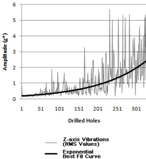
Figure 9: RMS values of the obtained vibrations and the related best fit curve (\*g=9.81 m/s<sup>2</sup>)
