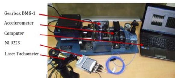
Fig. 1. Experimental gearbox and measuring system
