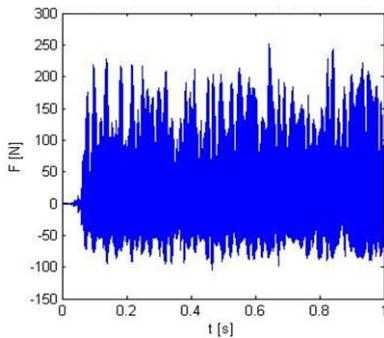
Fig. 8. Signal from model for correct work of the gears, with high loading and rotational speed 800 RPM
