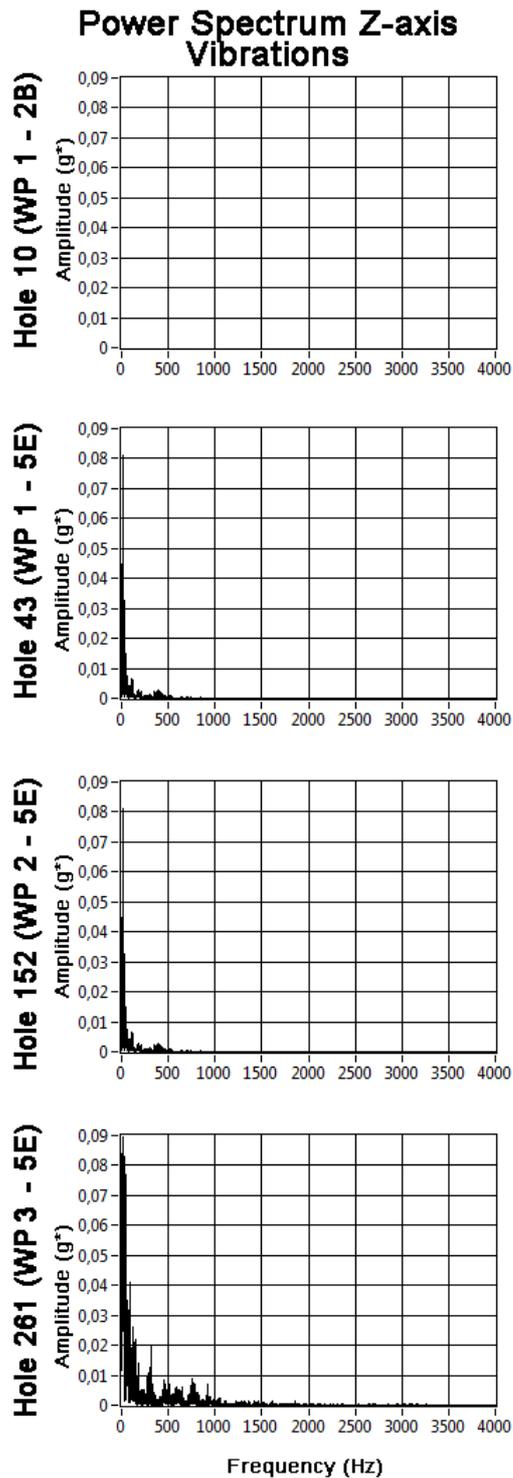
Figure 13: FFT analysis of the obtained vibration signals (\*g=9.81 m/s<sup>2</sup>)
