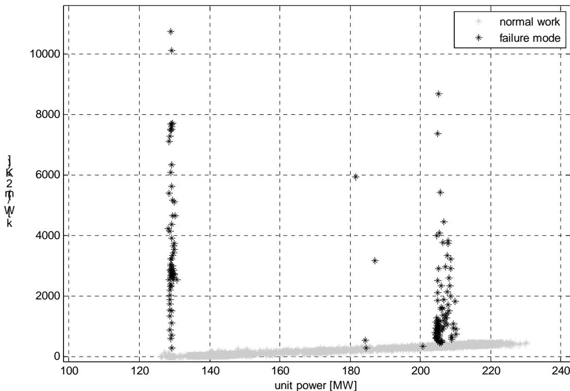
Fig. 5. Heat transfer coefficient versus unit power during normal operation and failure mode
