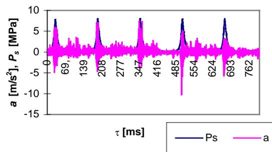
Fig. 2. Time courses: of accelerations vibration signal processed on the screw of the cylinder head and in-cylinder pressure of marine engine by the pressure sensor fastened on the indicator valve:  $a$  – acceleration vibration,  $P_s$  – in-cylinder pressure,  $\tau$  – time
