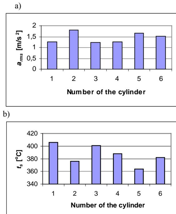
Fig. 8. The root-mean-square values accelerations vibrations  $a_{rms}$  (a) interdependent with the maximum combustion pressure in the individual cylinders and value of the exhaust outlet temperature  $t_s$  (b) for the individual cylinders
