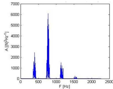
Fig. 11. PSD for signal from model for incorrect work due to misalignment of the gears, with high loading and rotational speed 800 RPM
