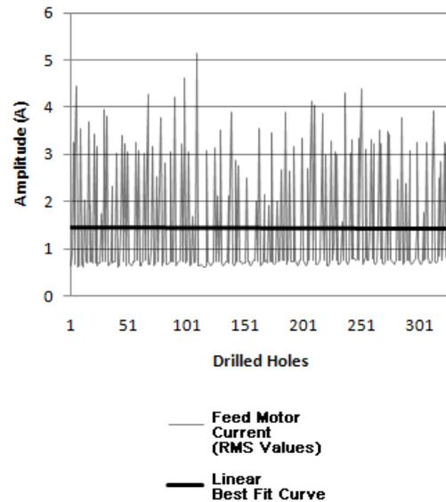
Figure 12: RMS values of the measured feed motor and the related best fit curve
