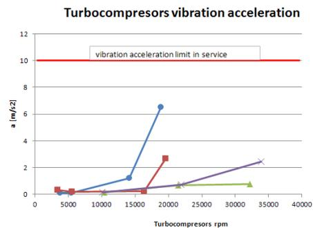
Fig. 11. I-th harmonic vibrations acceleration amplitude measured on turbochargers bearing casing versus turbocharger rpm SG LB (blue line) – main engine port side, SG PB (red line) main engine starboard, ZP 1 (green line) - Diesel Generator No. 1, ZP 2 (violet line) - Diesel Generator No. 2
