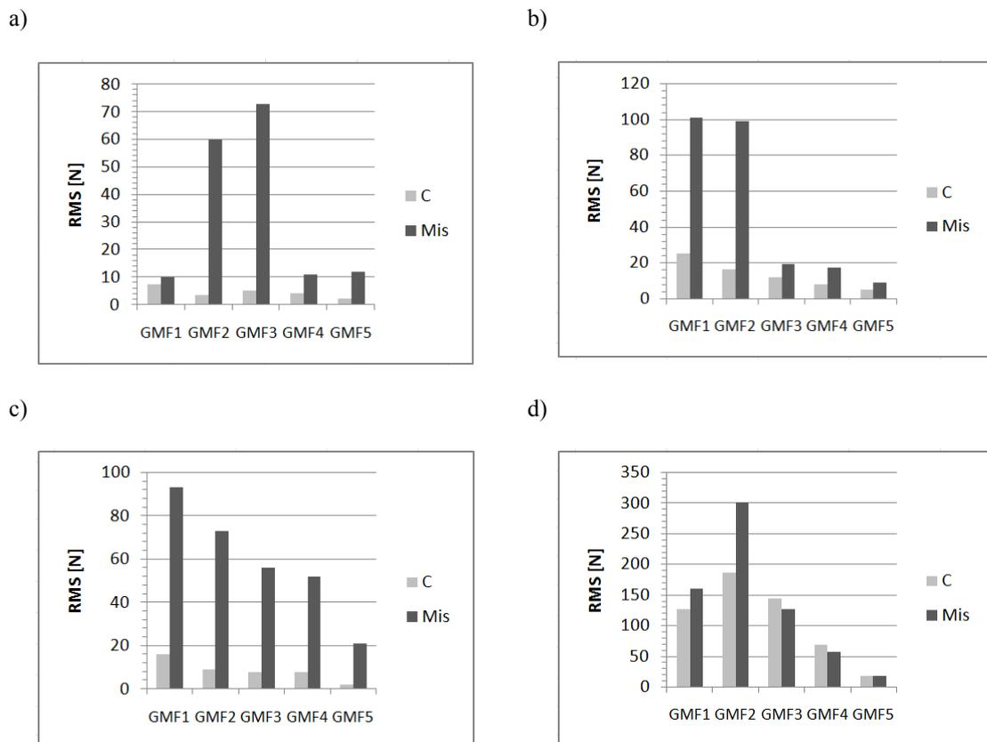
Fig. 13. RMS in bands for signals from model, a) 400RPM, low loading, b) 400 RPM, high loading, c) 800 RPM, low loading, d) 800 RPM, high loading. (C- correct state, Mis–misalignment)
