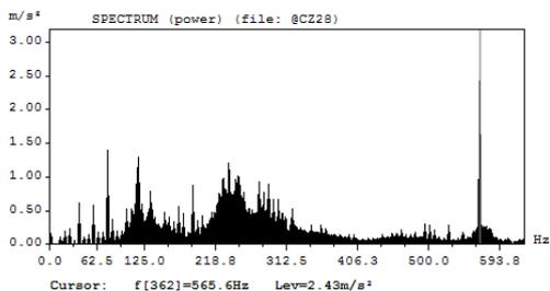
Fig. 8. Turbocharger amplitude of vibrations accelerations in frequency domain Diesel Generator No. 2
