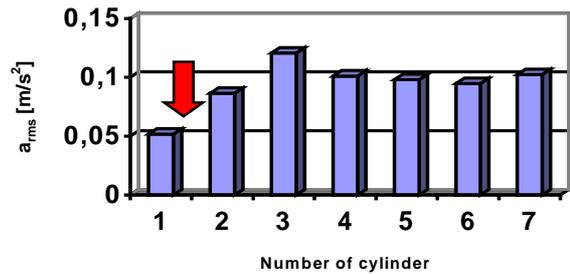
Fig. 9. Root-men-square values of accelerations vibrations signal by the sensor fastened on the cylinder head cover screws for 1–7 cylinders of 7L16/24 engine: ↓ – failed of piston-cylinder group after restart the engine
