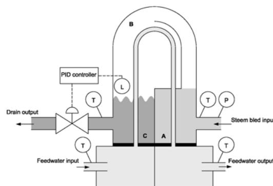
Fig. 2. Schematic representation of a three-zone feedwater heater [1] (A: desuperheating area; B: condensing area; C: subcooling area; T: temperature sensor; L: level sensor; P: Pressure sensor)
