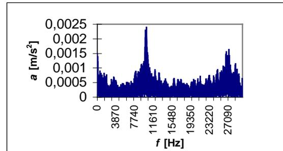
Fig. 5. Examples of the amplitude spectrum of accelerations vibration signal in the 0–30 000 Hz frequency band: rated engine speed 1200 rpm,  $f$ –frequency
