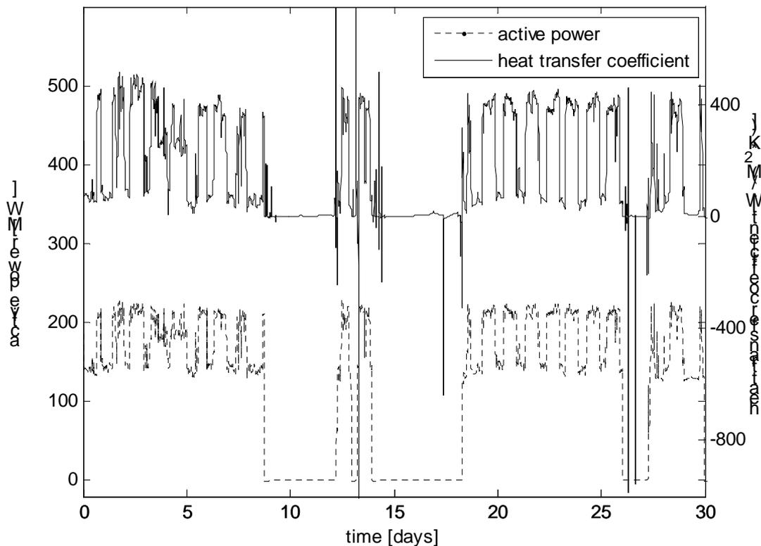
Fig. 4. Trends of heat transfer coefficient for heater XW1 and active power of the unit
