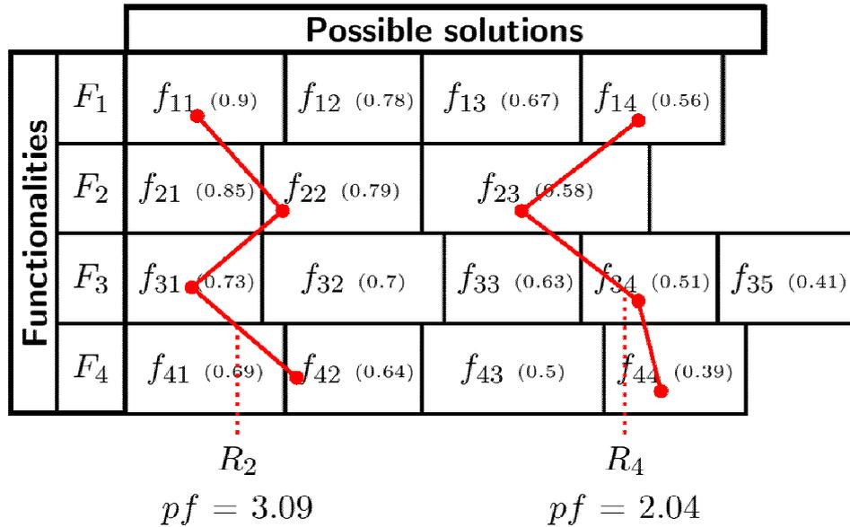
Fig. 6. Exemplary preference factors of particular elements of a morphological table (values in brackets) and selected solutions of a diagnostic system,  $pf$  – preference factor
