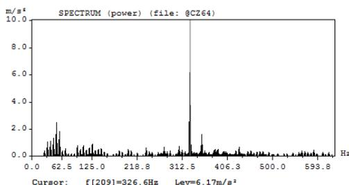
Fig. 4. Turbocharger amplitude of vibrations accelerations in frequency domain Main Engine – starboard side
