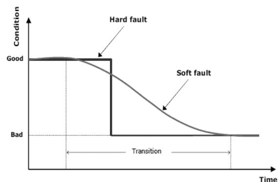
Figure 1: Hard and soft faults, Courtesy of [2]
