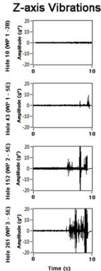
Figure 6: Raw Z-axis vibration signals for the time period of specific drillings (\*g=9.81 m/s<sup>2</sup>)
