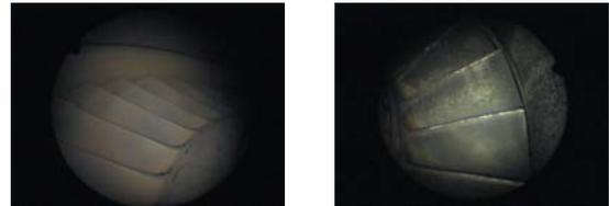
Fig. 6. Turbine (left) and compressor (right) wheels - Main Engine – starboard side
