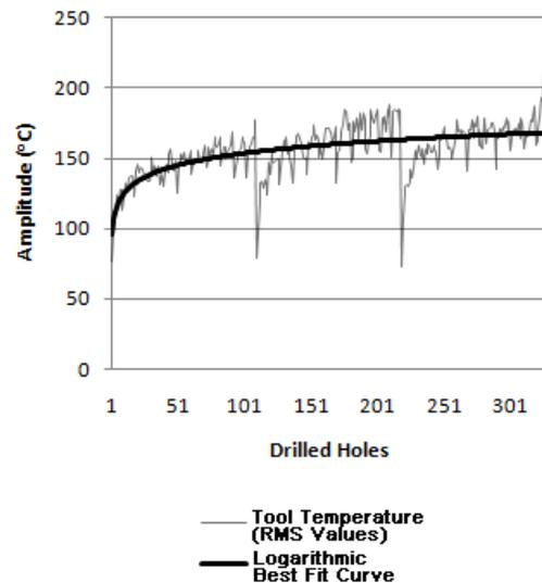
Figure 10: RMS values of the measured tool temperature and the related best fit curve
