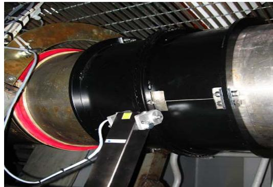
Phot. 1. Toothed rings and laser sensor ETNP-8 mounted at intermediate shaft
