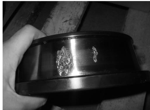
Fig. 4. Spalled inner race of a wind turbine
